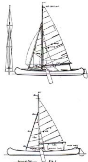
At top: Class B Canvas Canoe, sloop rigged. At bottom: Class C Canvas Canoe.
